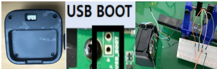
Figure 24: Attempt to connect debug port and serial port of kakao mini
